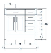
thin frames:  $\frac{3}{4}$  thick frame bottom: 2
